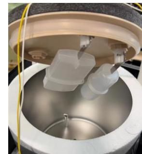
6. Add the recommended amount of an approved sanitizing agent to the water inside the cold tank and gently mix. Allow this mixture to sit in the tank for at least 10 minutes. After 10 minutes has passed, position a bucket or large container under the white drain cap on the back side of the unit. Remove the cap to this drain port and allow the sanitizing agent and water mixture to drain into the bucket. With a pitcher ready, dispense cold water until the tank is empty.
