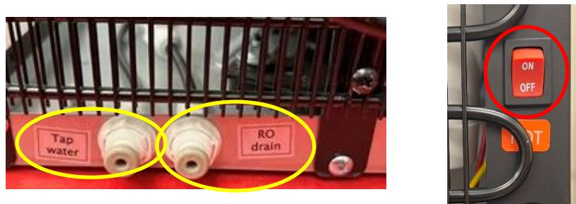
2. If not already done during the filter flushing process, remove the right-side panel of the unit. Two screws down at the bottom of the panel must be removed. Then, lift the lower lip of the panel and pull outward. The panel should hinge outward, and then come away from the unit completely. Set this panel aside. Turn the water to the unit on.
