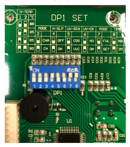
To disable the energy saver, DIP #4 must be switched from ON to OFF.
