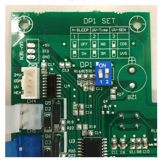
To disable the energy saver, DIP #1 must be switched from ON to OFF.
