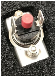
← CLOSE UP OF THE MANUAL OVERLOAD
