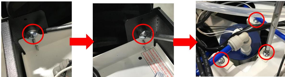
Lift the Firewall assembly off the white shelf and pull the front panel away from the machine. Without disconnecting any wiring, slightly pull the panel away from the front of the machine, enough to give room to fit your hand inside the front of the machine. Locate the Overload Thermostat on the front of the Hot Tank (has a bright red button on it). Reach in and depress the red button in the center of the thermostat to manually reset the Overload Thermostat.
